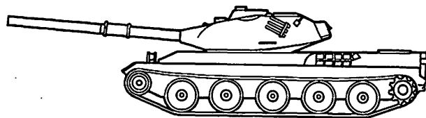
ST-8-JAPANESE TURTLE SHAPED TURRET, FORWARD OF CENTER 5 ROAD WHEELS, NO SUPPORT ROLLERS VARIABLE SUSPENSION SMOKE LAUNCHERS ON BOTH SIDES OF TURRET
